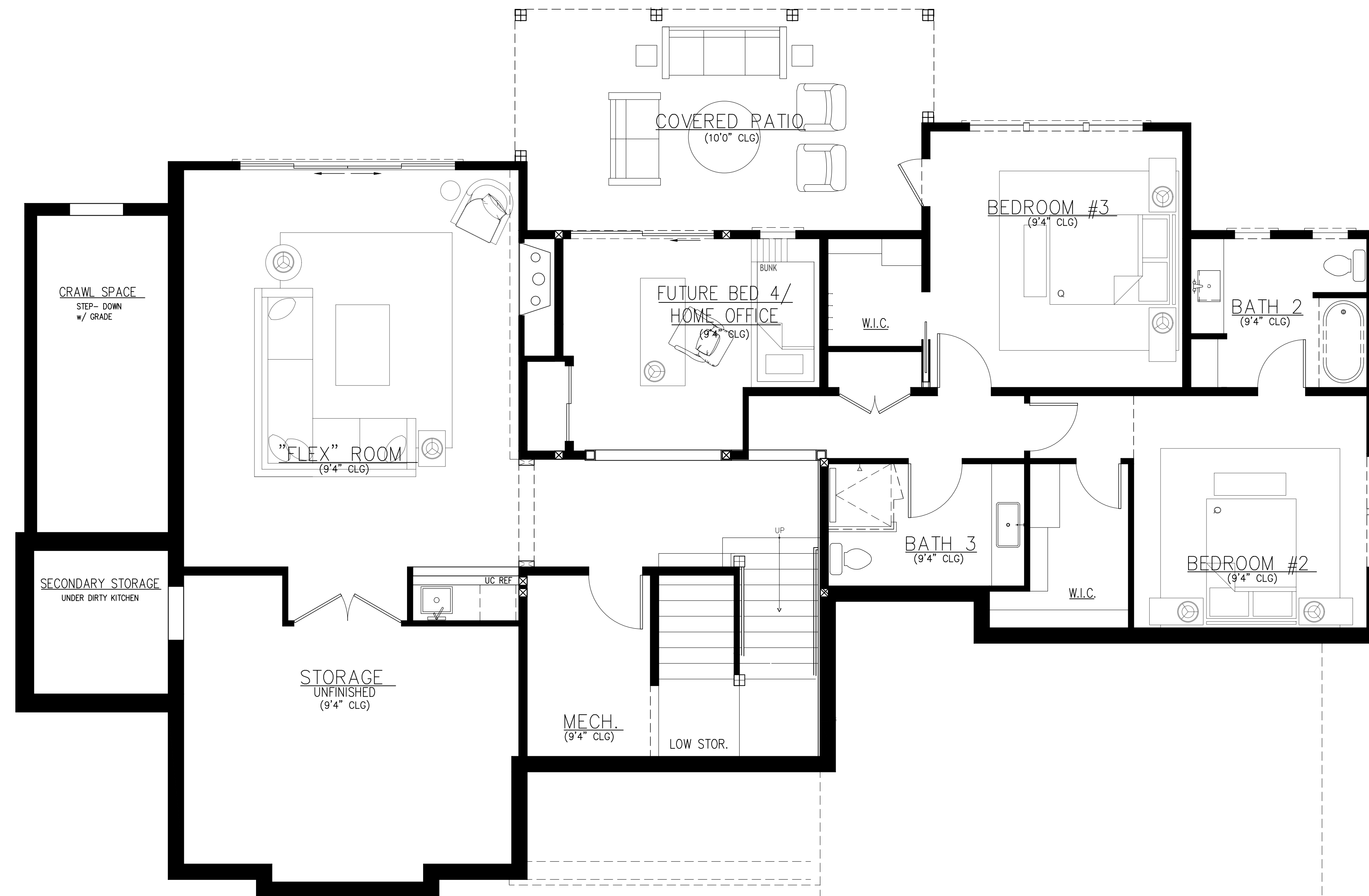
1 LOWER LEVEL FLOOR PLAN SCALE: 1/4" = 1'-0"
